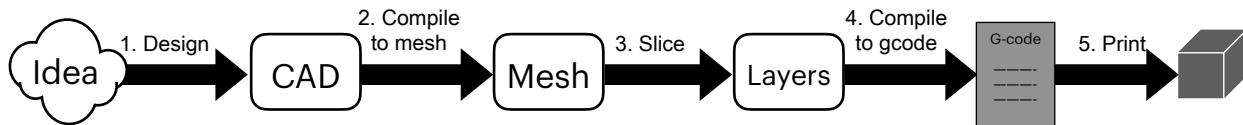
Figure 1: A typical 3D Printing Workflow. Once a model is designed using CAD tools, it is compiled down to a polygon mesh. The mesh is then sliced to generate 2D layers. The layers are then compiled to G-code. Ultimately, the G-code is sent to a printer which has firmware that can interpret the G-code to print the model.
