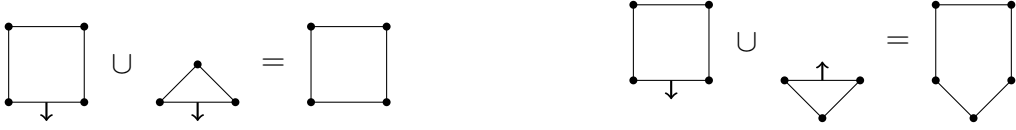
(a) Keeping a common edge during mesh union. (b) Removing a common edge during mesh union.
